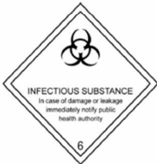
Figure 1b. Hazard label for Category A infectious substances and for genetically modified microorganisms and organisms that meet the definition of an infectious substance, Category A.
